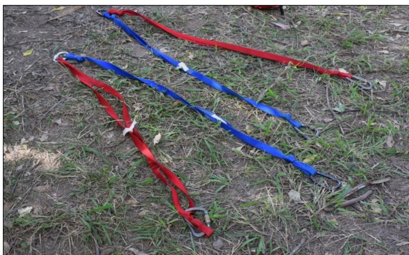
Figure 1: Example of two sets of lanyards similar to those in use at the time of the incident.
